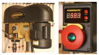
The full 1 HP motor (left) and control panel (right) make controlling the PM2800 for your job easy. The green pilot light in the center of the red pull On, push Off button is an indication that the PM2800 is connected to electrical current.
